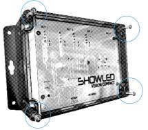
1. Open 4 screws that are holding the transparent cover and remove the cover.
